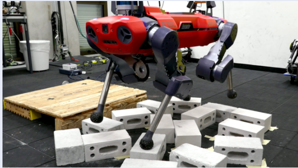
FIGURE S14 Control barrier function (CBF) safety filter on a quadruped. A multilayered safety filter design is used that integrates predictive safety filters with CBFs to ensure safe foot placement on viable footholds while maintaining system stability. CBF constraints are integrated into both a mid-level predictive filter and a low-level CBF based filter given by (29), ensuring a consistent safety specification across planning and control layers [88].
