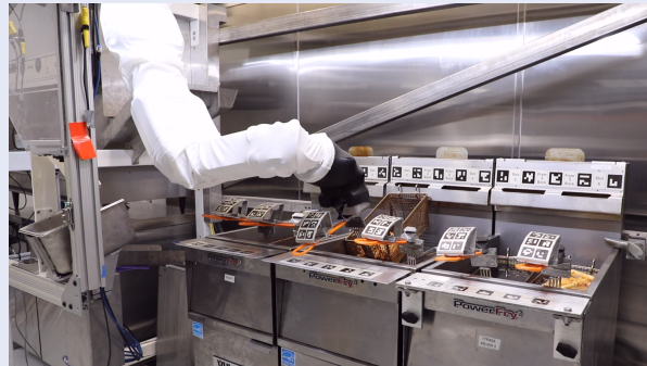
FIGURE S16 Control barrier function (CBF) safety filter on a robotic arm in an industrial kitchen. Maintaining safety in a dynamic work environment shared with human personnel requires online modification of arm reference trajectories, but directly recomputing trajectories online is computationally intractable for real-time operation. CBF-based safety filters are used to efficiently modify trajectories given ongoing changes in the environment. [86].
