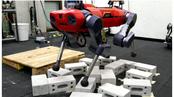
Fig. 1. ANYmal [6] performing a trotting gait on stepping-stones.
