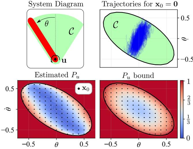
**Fig. 3. (Top Left)** System diagram of the inverted pendulum. **(Top Right)** 500 one second long example trajectories starting at  $\mathbf{x}_0 = 0$ . **(Bottom Left)** Monte Carlo estimates of  $P_u$  for  $\gamma = 0$  using 500 one second long trials for each initial conditions represented by a black dot. **(Bottom Right)** Our (conservative) theoretical bounds on  $P_u$  from Theorem 5
